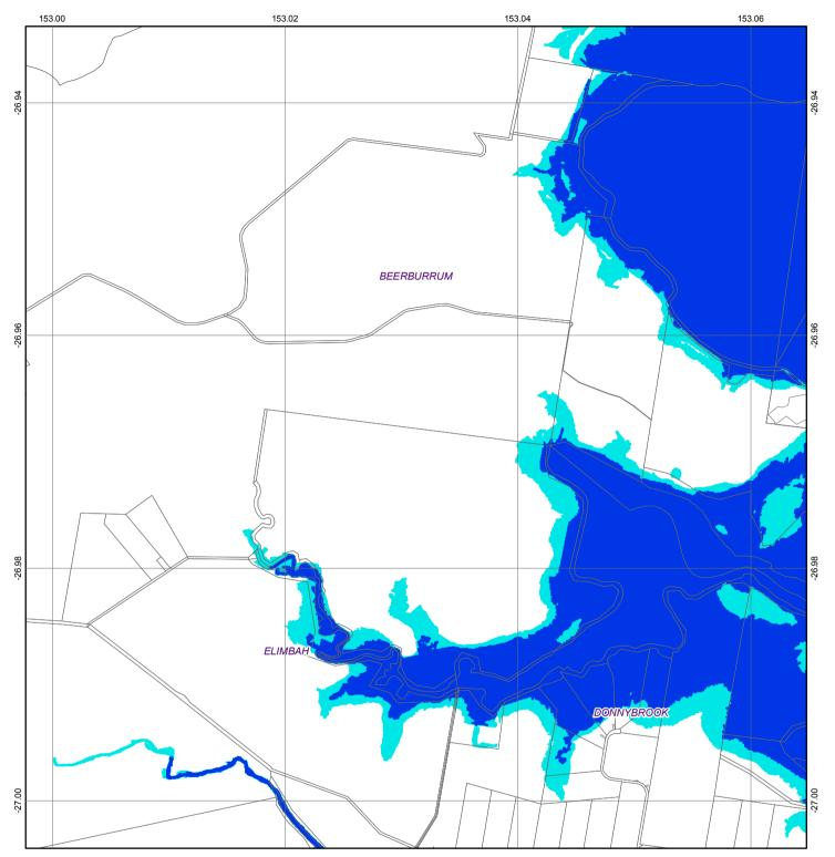
1. A default storm tide inundation level of 1.5 m HAT in South East Queensland regional planning area and 2.0 m HAT for the remainder of Queensland is used where projected storm tide inundation levels have not been determined locally. The default level uses a sea level rise factor of 0.8m to 2100.
